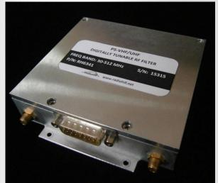
The preselector RH6341 is digitally tunable filter operating from 30 MHz to 512 MHz. This module consists of three (3) internal tunable bandpass filters (the frequency range divided between them in the following way: 30-96 MHz, 96-262 MHz and 262-512 MHz). RH6341 uses serial or parallel interface for tuning.
