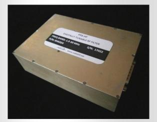
The RH6331 is digitally tunable filter operating from 30 MHz to 88MHz. Parallel interface is used for tuning. The module can be installed either in receiving or transmitting tract. RH6331 has low insertion losses, high RF power handling, wide operating temperature range and fast tuning speed. The module can work in frequency-hopping spread spectrum mode.
