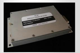
The preselector RH6323 is digitally tunable filter operating from 1.5 MHz to 30 MHz. This module consists of two (2) internal tunable bandpass filters (the frequency range divided between them in the following way: 1.5-6.7 MHz and 6.7-30 MHz) and the internal amplifier (it compensates filter's insertion losses). RH6323 uses serial interface for tuning.
